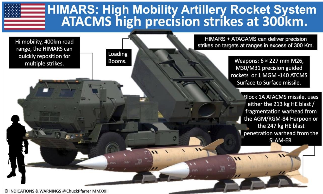
Figure 2: AGM-140 ATACMS missiles on display in front of a HIMARS launch vehicle
